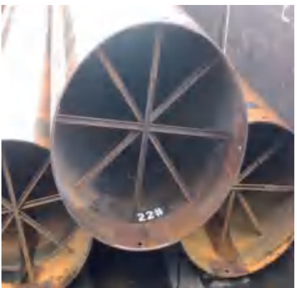
7.Cross Bar Welding
