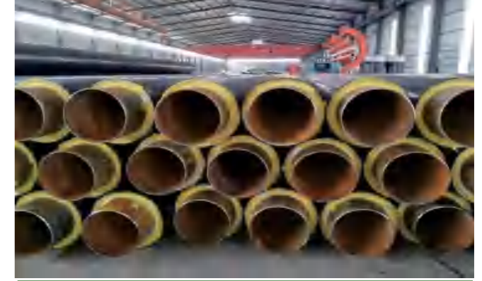
6, Thermal Insulation Coating
